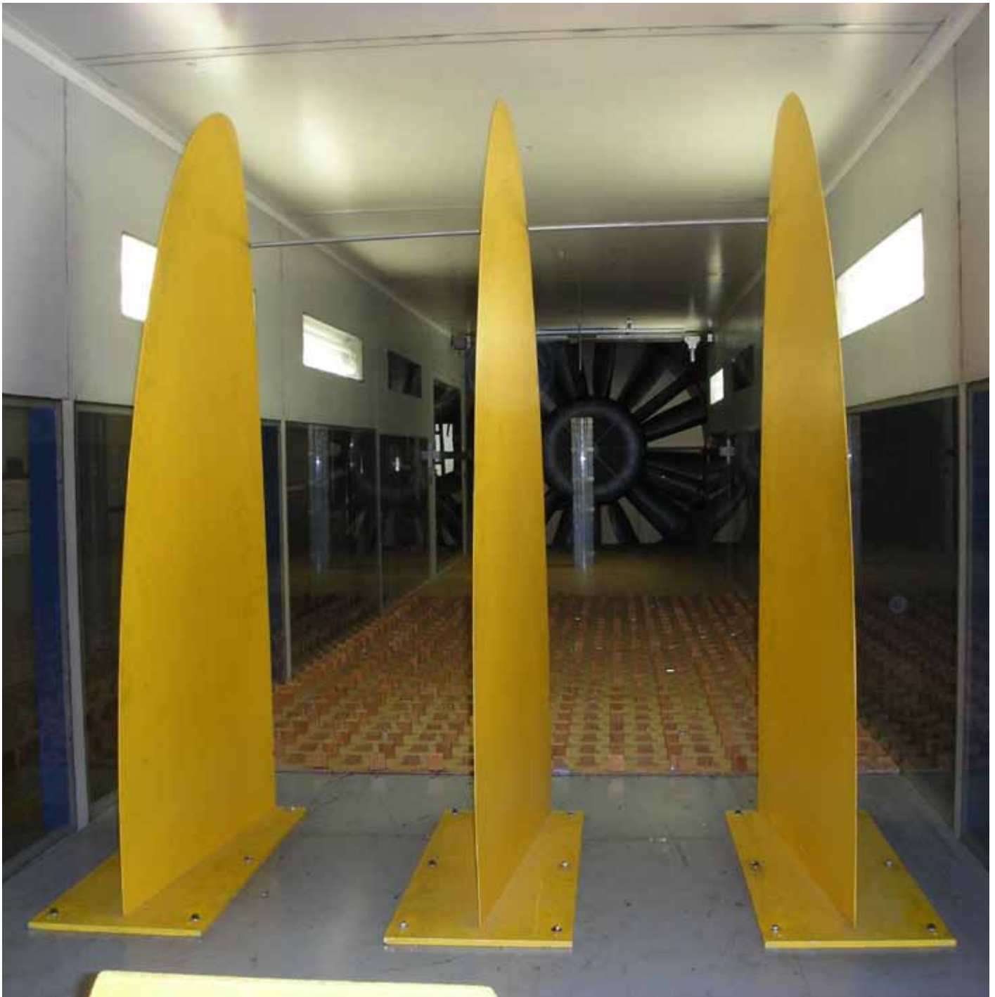
Figure 8: View of the model in wind tunnel
